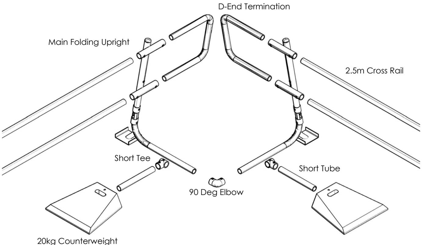
Begin by assembling a complete corner unit consisting of two folding uprights, two counterweights, two d end terminations, two short tee's and a 90 deg elbow.
